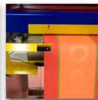
Optical edge alignment sensor ensures that reference edge of fabric is kept aligned to ensure perfectly straight, rectangular cuts.
