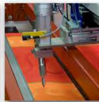
Ultrasonic cutting on both length and cross cuts provides clean, sealed edges. Integrated optic sensor measures fabric width so that cutting dimensions are automatically calculated.
