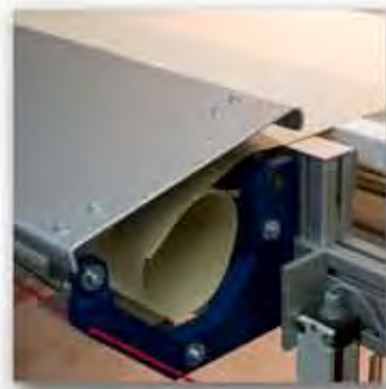
Optional high speed fabric re-winder rolls cut pieces onto one another without wrinkles. Panels are rolled lengthwise ready for seaming operation.
