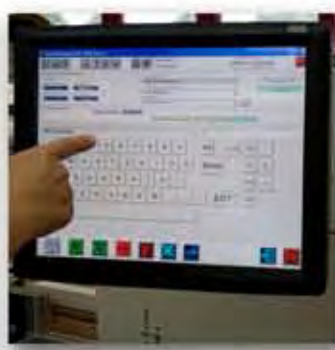
Operator friendly Touchscreen allows direct entry of finished awning dimensions on graphic display.
