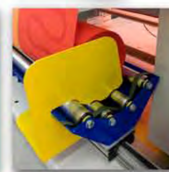
Fabric roll is automatically secured to prevent roll drift during fabric pulling.
