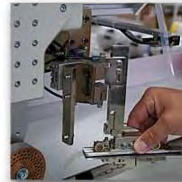
Application specific guiding devices ensure precise, consistent seams. A pneumatic "quick-change" mechanism allows these to be changed in seconds to maintain high machine throughput.
