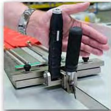
Material is pre-tensioned as required with a precision adjustable clamp / torque applicator, ensuring the required tension is applied by every operator, every time.
