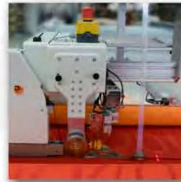
The welding head travels while the material is clamped in the work table. Precise synchronisation of the head travel, sonotrode rotation, and anvil rotation is maintained to ensure flat seams. As the material passes between the rotating sonotrode and anvil wheel, it is welded or glued using heat activated adhesive film.
