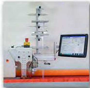
Ultrasonic head, Touchscreen, and material guides with adhesive film feed are located in close proximity to provide an efficient workspace. All machine setup parameters are stored and easily recalled and implemented from the control unit.
